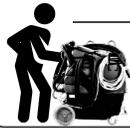
Fill rescue machine with water from a janitors sink, bucket or using the available sink adapter hose.
